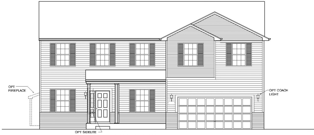
4" HORIZONTAL SIDING, BRICK FRONT ELEVATION "B"
