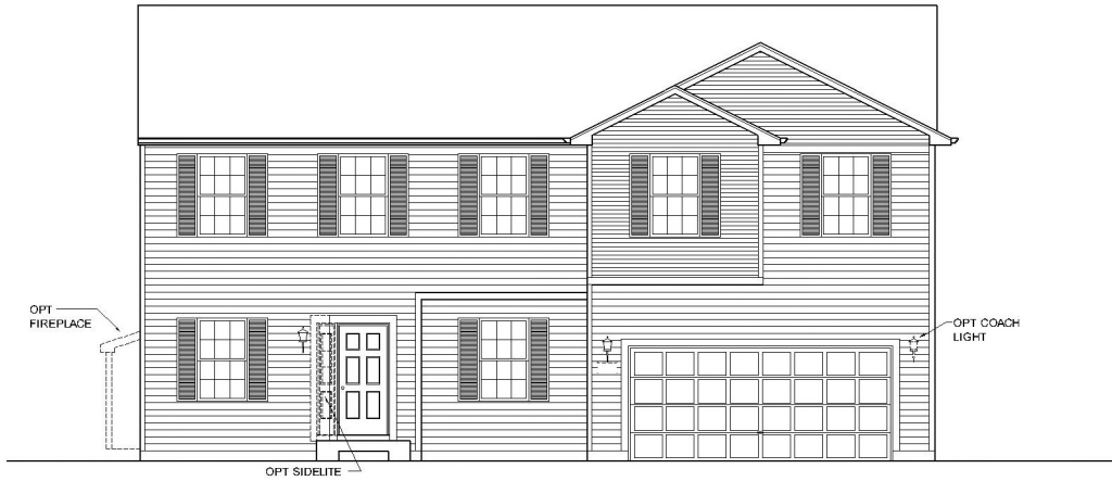
4" HORIZONTAL SIDING FRONT ELEVATION "A"
