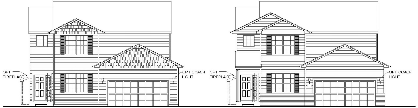
HORIZONTAL SIDING, SHAKES FRONT ELEVATION "A"
