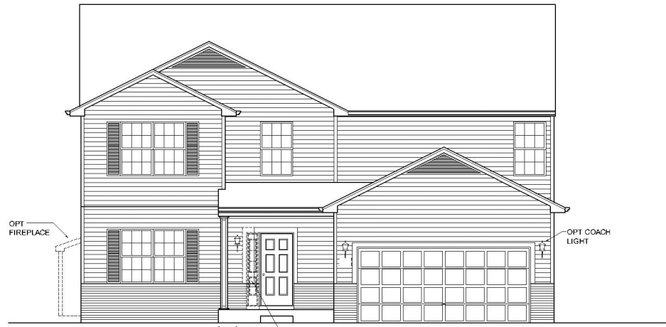
4" HORIZONTAL SIDING, BRICK FRONT ELEVATION "B"
