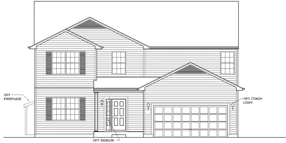
4" HORIZONTAL SIDING FRONT ELEVATION "A"
