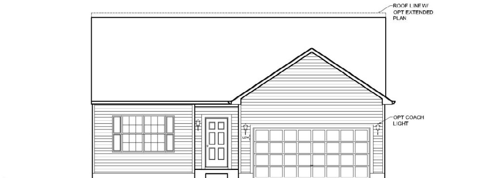
4" HORIZONTAL SIDING FRONT ELEVATION "A"
